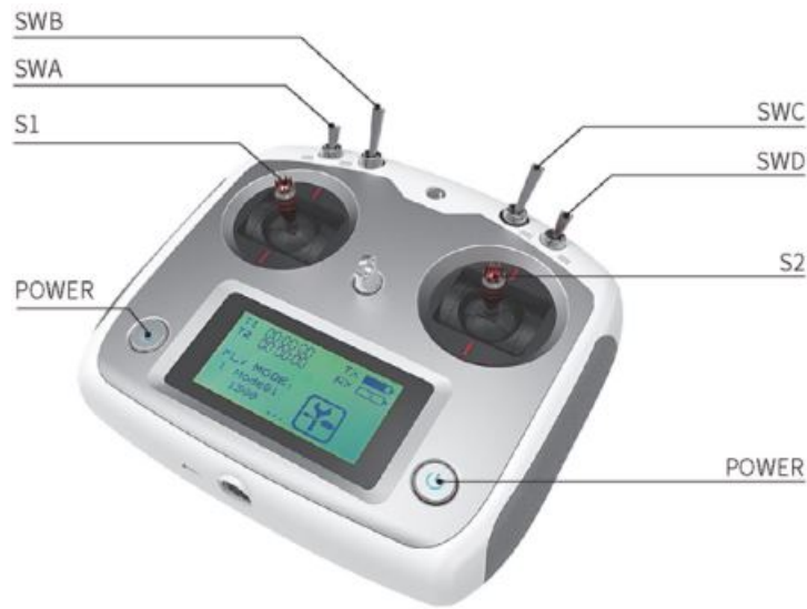
Figure 2.3 Schematic diagram of FS remote control buttons
