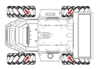
Note: Make sure that each Mecanum wheel is installed at the right angle as shown above.
