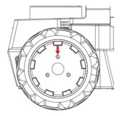
2. Align the holes to install the hubcap, and tighten the M3\*12mm screws.
