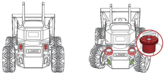
2. Switch to four-wheel differential mode(yellow light):
