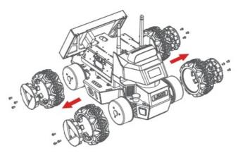
2. Install the Mecanum wheels with the M3\*5 screws in the package. Switch to the Mecanum mode through APP, when the LIMO indicator light turns blue, the switch is successful.
