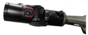
2. Solid green light: The robotic arm has entered the drag & teach mode for trajectory recording.
