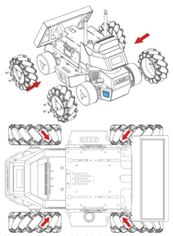
Note: Make sure that each Mecanum wheel is installed at the right angle as shown above.
