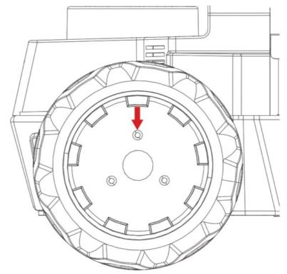
2. Align the holes to install the hubcap, tighten the mounting gear, and wear the tire on; M3'12mm screws.
