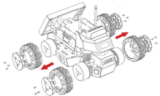
2. Install the Mecanum wheels with the M3'5 screws in the package. Switch to the Mecanum mode through APP, when the LIMO indicator light turns blue, the switch is successful.
