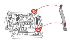
2. Loosen the screws shown in fig.4 and remove the plates.
