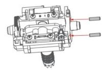
4. Place the spring hook assembly into position and hook the spring onto the hook located inside the transmitter.
