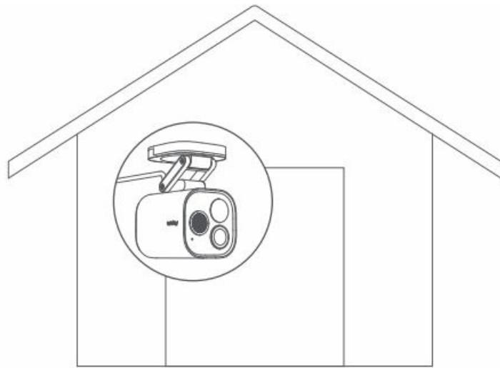
2. Loosen the fastening screws of the wall mounted bracket, take out the bracket, attach it to the selected installation position on the wall, and mark the punching points.
