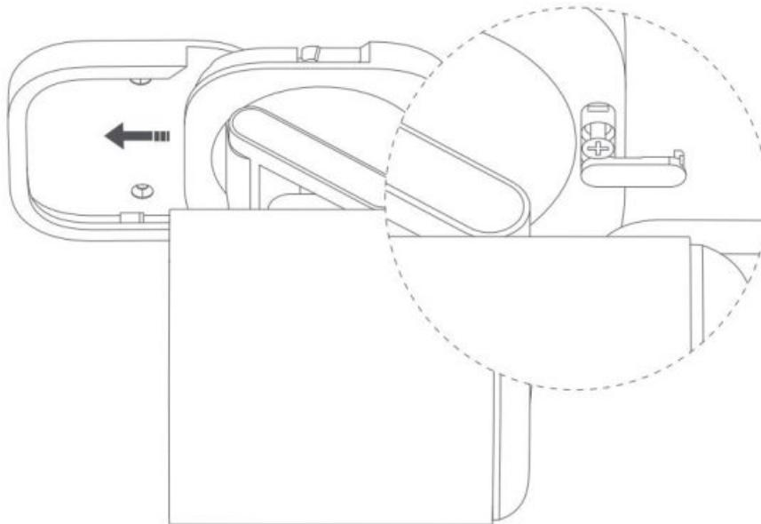
8. After successfully adding the camera to the App, manually adjust the pitch angle or left and right rotation angle of the bracket based on real-time video, and aim the lens at the position that needs to be photographed.
