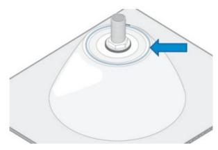
5. Apply the silicone slightly in from the edge of the outer edge of the underside of the basin
