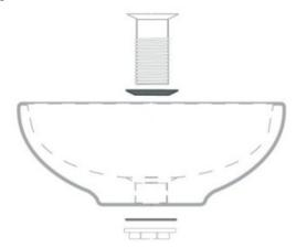
4. Apply a bead of silicone slightly in from the edge of the basin
