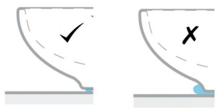
6. Place the basin into position with the waste through the drilled hole Allow all sealant to dry for at least 24 hours before use
