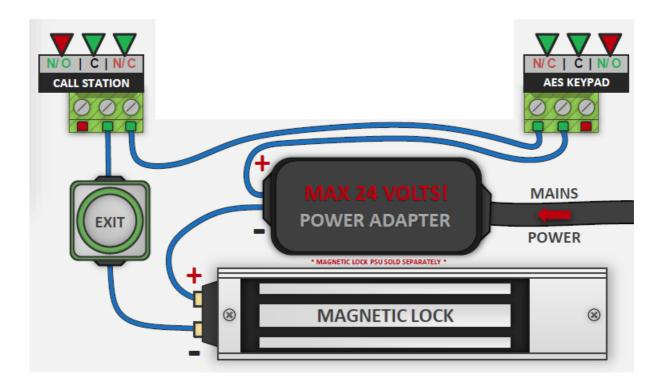
Follow this method when using a magnetic lock. If the relay in either the Call Station or optional AES Keypad is triggered it will temporarily lose power and allow the door/gate to release. For installs without the optional AES Keypad; connect the POSITIVE of the Magnetic Lock PSU to N/C terminal on Call Station Relay
