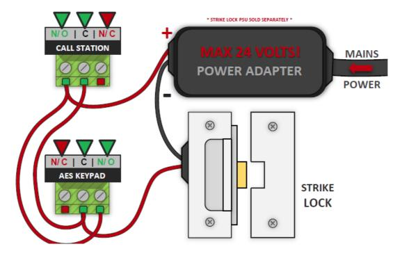
Follow this method when using a Strike Lock with the system. If used it will mean that if a relay in either the Call Station or optional AES Keypad is triggered it will temporarily allow the door/gate to release.
