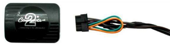
3. Connect the opposite end of the head unit patch lead to the head unit steering wheel control input on the back of the aftermarket head unit.
