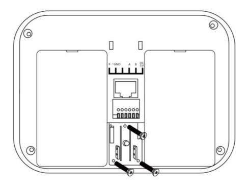
**Step 4**Mount the larger bracket onto the wall and secure it with screws
