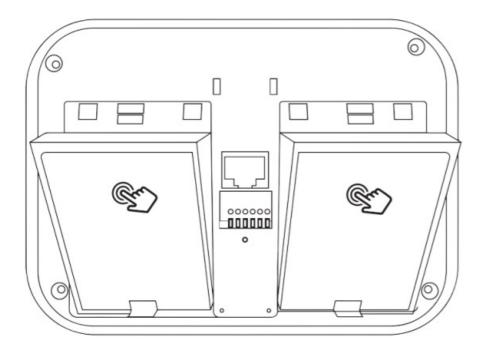
**Step 2**Position the cover over the capsules and press down firmly on the upper part to ensure a secure ft.
