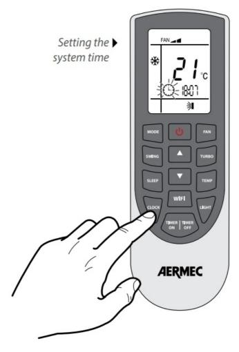
These units are equipped with an internal clock which can display the current time; by pressing on the key the clock icon will start to flash (this flashing will last 5 seconds, after this if no key is pressed you automatically exit the time modification mode); while the clock icon is flashing it is possible to change the system time using the keys and to increase or decrease the displayed time; once the desired value is set you need to wait 5 seconds or
