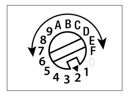
15 indexation positions are allowed for Modbus addressing: position 1 to position F included. Address 0 is not available.
