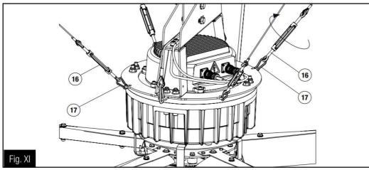
Connect the Ø3mm stabilizing wires with turnbuckle (16) to the motor support using the 5mm snap-hooks (17) and stabilise the fan; securely fix the other end of the stabilizing wires to the ceiling using the clamps (18). Fixing screws for the ceiling/beam are not supplied.
