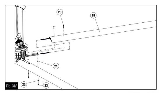
Insert the blade (19) over the blade root, lock it with the M8 flange bolts (20), spring washers (21) and locknuts (22). Tighten the screws making reference to table 1. Mount the plastic caps (23) on the locknuts.
