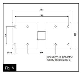
• Fix the downrod (6) to the ceiling brackets (7) by means of the M12 bolts (8), the flat washer (9), the spring washers (10) and the locknuts (11).
