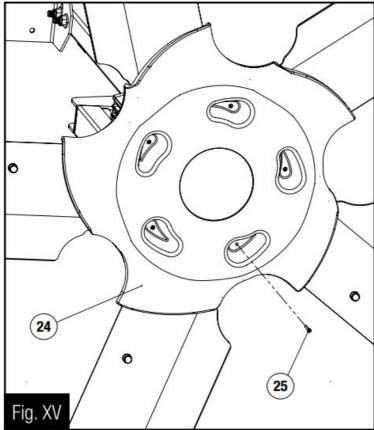
Mount the plastic cover (24) under the hub using the M4 bolts (25); in case water is used for washing, drill a hole in the plastic cover for water drainage.
