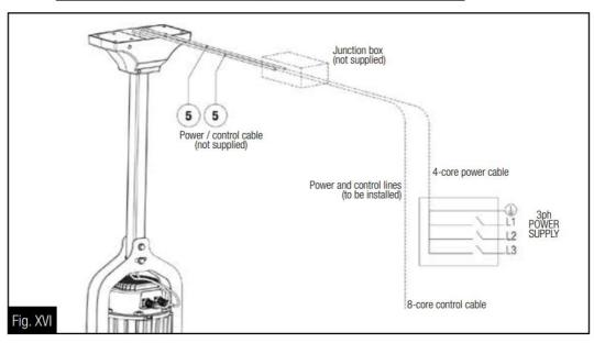
Make the connection to the power supply/control network by connecting the wired cables to the motor (5) through a junction box (not supplied) to be placed near the ventilation unit. Size the cables appropriately taking into account the distance between the ventilation unit and the power supply The complete electrical system must be carried out by a qualified and authorized installer, in accordance with the local requirements.
