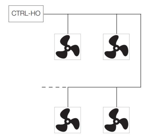
If the units are not connected as per the diagram above, a degradation of the communication signal may occur and the network may not function properly.
