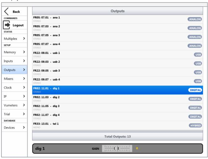
For each output, module type (for example, digital FR02 or hybrid FR33), slot number (for example, 11), channel number within that slot (for instance, 01), output's logic name (for example, dig 1), signal type (for example, DIGITAL) and signal channels number (for example, STEREO) are displayed.
