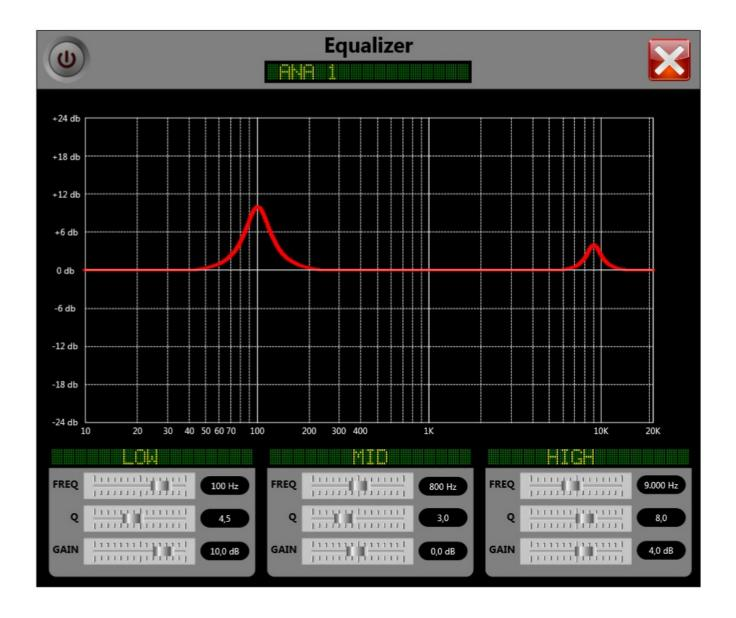
Once inside that configuration screen (equalizer in the example), in addition to modify the process associated parameters, the **ON/OFF button** (at the top left area) allows you to activate/deactivate the process and the button (at the top right area) allows you to return to the previous screen (or simply by clicking on the graphical representation).
