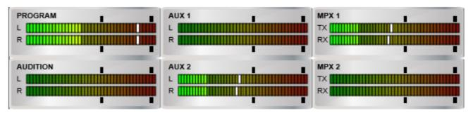
The "PROGRAM" and "AUDITION" vu meters are always displayed, whereas the rest of them are only shown when no channel is selected by means of the button
