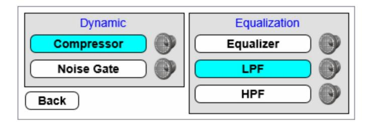
In order to activate/deactivate a process, just click on the button with its name. When the process is active, it will appear with a blue background, otherwise the button will have white background.
