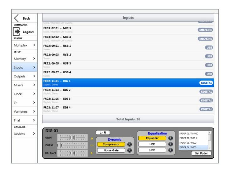
For each input, module type (for example, digital FR02 or hybrid FR33), slot number (for example, 11), channel number within that slot (for instance, 01), input's logic name (for example, DIG 1), signal type (for example, DIGITAL) and configuration details (for example, Digital / Stereo) are displayed.
