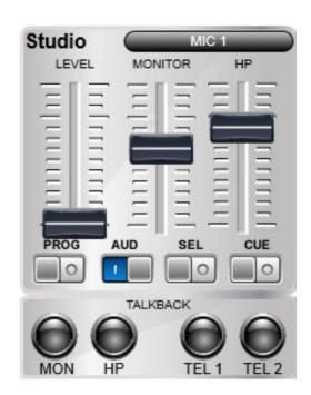
The CUE vu meter (or the control monitoring bus vu meter, when there are no channels sent to CUE), together with a button implementing the "CUE RESET" function, are displayed in the Control section. This button operates in parallel with the one programmed in the programmable keys section.
