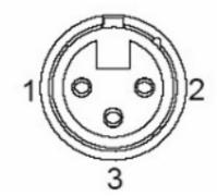
Pin 1: Ground Pin 2: Input + Pin 3: Input –
