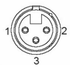
Pin 1: Ground Pin 2: Input + Pin 3: Input –
