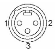
Pin 1: Ground Pin 2: Output + Pin 3: Output –
