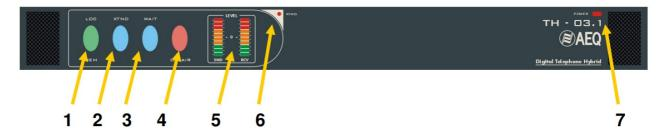
1. "LOC/REM" key: allows you to change between local (without pressing) or remote control (pressed). Both modes are exclusive between them.
