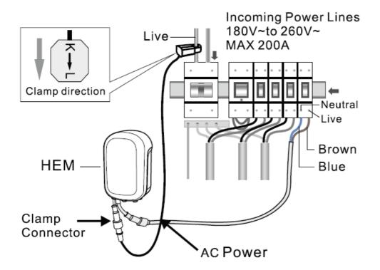
In 230 volt countries with a 3 phases and 3 wires installation;
