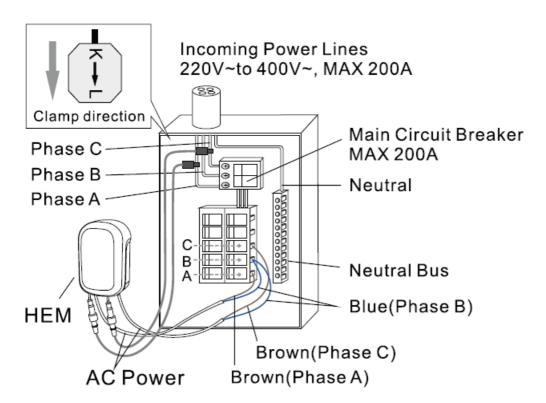
In 230 volt countries with a 3 phases and 4 wires installation;
