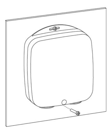
2. Loosen your Heavy Duty Smart Switch's lower screw to release its shell. Remove the shell to reveal the inner electronics:
