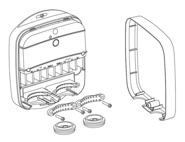
3. Prepare the wires you will be attaching to your Heavy Duty Smart Switch by stripping them to the necessary length. Add wire terminals to each wire.
