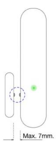
For German styly windows there the window sits on top of the windo frame mounting on the side of the window is highly recommended. If no tilting detection is used, the sensor can be placed on any position of the door or the window. In case tilting detection is desired the sensor should be placed on the upper side of the window.
