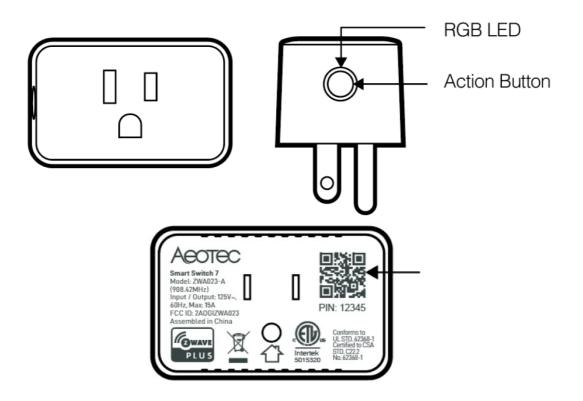
**Note:** QR Code used for SmartStart inclusion. DSK Code can be found on the packaging. Do not remove or damage them.
