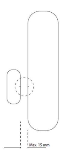
• The standard magnet covered by the plastic part, mountable beside the sensor. Make sure the two indicating lines on sensor enclosure and magnet are opposite to each other. The image on the right-hand side shows the
