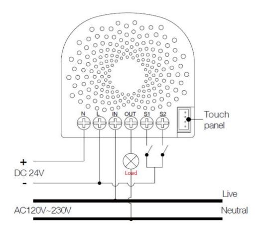
Note: The ?IN? terminal should be connected to the ?Live? of AC 120V/230V power wire.
