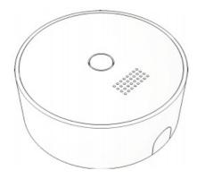
Popp 433 MHz Bridge has been crafted to connecting 433 Mhz devices with PoppHub or other compatible Gateways. It is powered by Popp Z-Wave technology.
