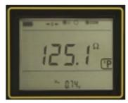
3. Press TEST. After a few moments, the reading appears. This should be  $25\Omega \pm 0.35\Omega$ .
