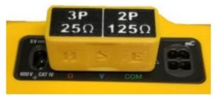
2. Observe the reading. This should be  $125\Omega \pm 2.7\Omega$ .
