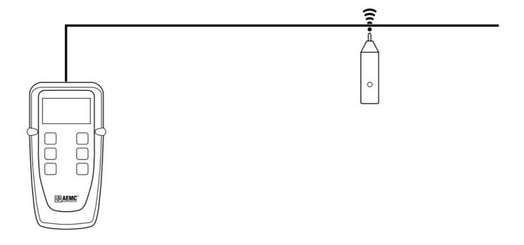
Pressing the TDR / button will inject a warbling (oscillating) tone into the cable or link under test. When set, the following will be displayed:
