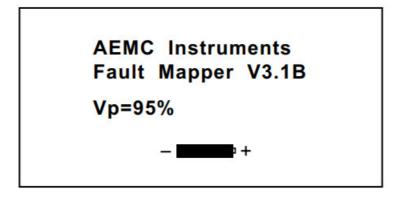
NOTE: When the Fault Mapper is turned off, it will remember the last selected Cable Library or Vp setting. This feature is useful in the situation where the operator is performing many tests on the same type of cable.
