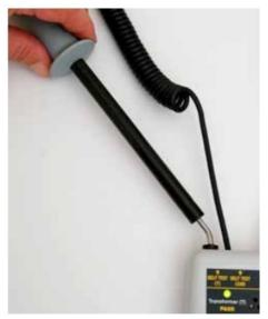
7. Insert the probe into the terminal labeled SELF TEST (C), and press TEST. The green Capacitor (C) PASS light should blink, and the buzzer should sound.
