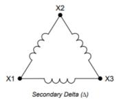
For Delta configurations, you must measure from each phase to other phases. Note that in this configuration, if one coil is open, the Model 8505 can still perform tests because the other two coils may be intact and there is a complete pathway
