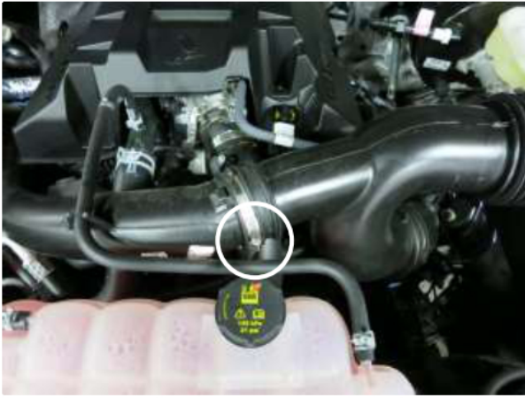
c. Loosen the hose clamp at the upper air intake tube.
