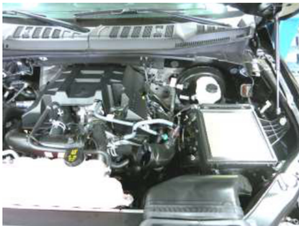
e. Remove the stock air intake system from the vehicle. Note: Do not discard any of your stock equipment.
