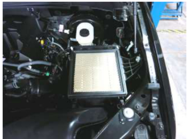
f. Remove your stock air filter from the lower air box.
