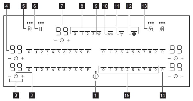
Use the sensor fields to operate the appliance. The displays, indicators and sounds tell which functions operate.
