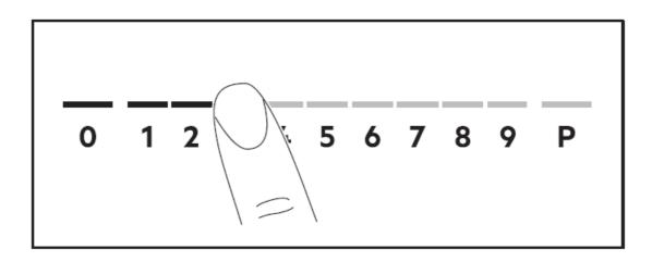
Press the desired heat setting on the control bar.
