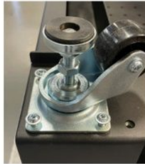
Figure 2.3 – Leveling pads on System's Wheels
