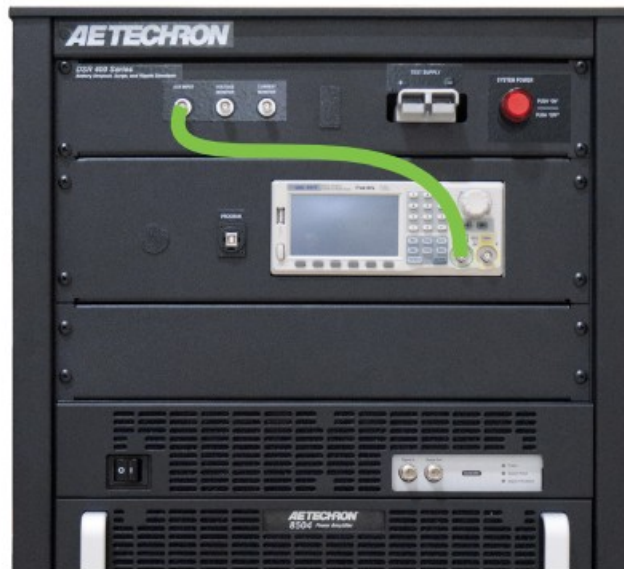
Figure 2.6 – Connecting for Signal Input from the Siglent SDG2042X
