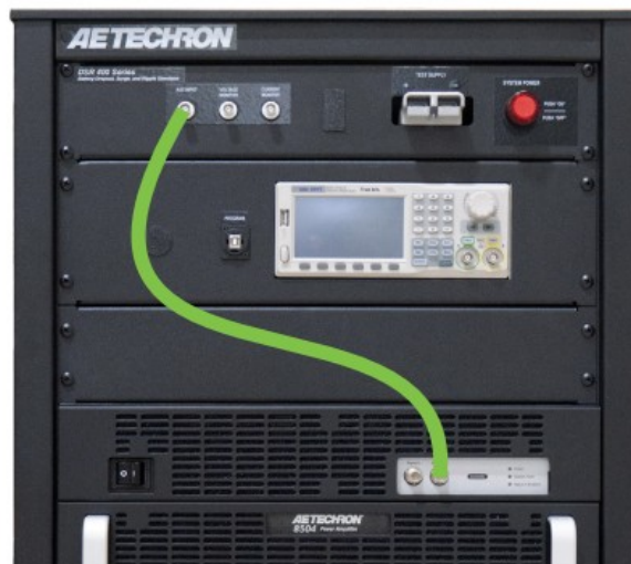
Figure 2.5 – Connecting for Signal Input from the AE Techron 3110A
