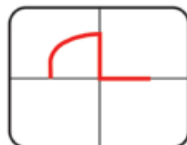
Figure 5.15 – Square Wave Showing an Increase in R is Required
