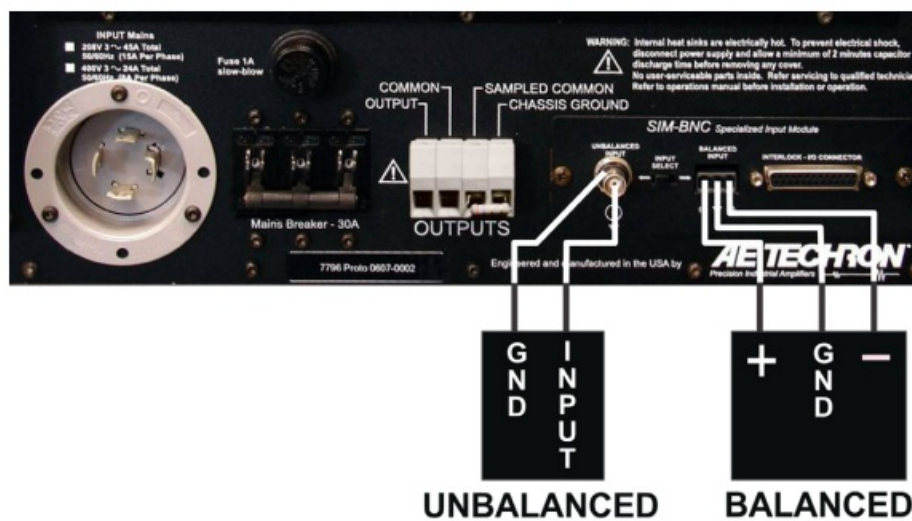
Figure 2.11 – Wiring for unbalanced or balanced input connector
