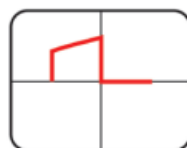
Figure 5.16 – Square Wave Showing an Increase in C is Required
