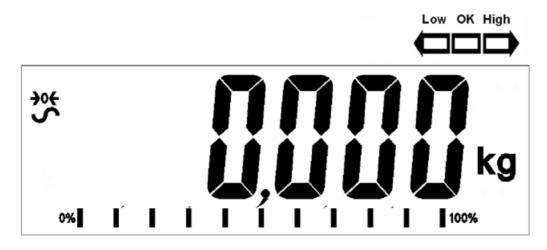
• The scale has an automatic re-zeroing function to account for minor drifting or accumulation of material on the platform. However you may need to press the **[Z/T]** key to re zero the scale if small amounts of weight are shown when the platform is empty.
