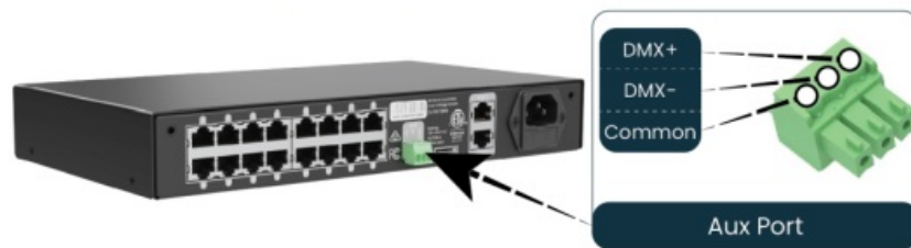
Figure 13: Location and Pinout of the Aux Port
