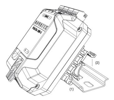
3. To remove the receiver from the DIN rail, pull the receiver horizontally, toward its power connector (1) and rotate the receiver up and off the rail (2), as shown in Figure 4 below.
