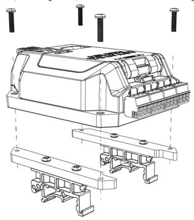
2. Align the lower edge of the bracket with the lower edge of the DIN rail (1), and push the receiver down so it clicks onto the DIN rail (2), as shown in Figure 3 below.
