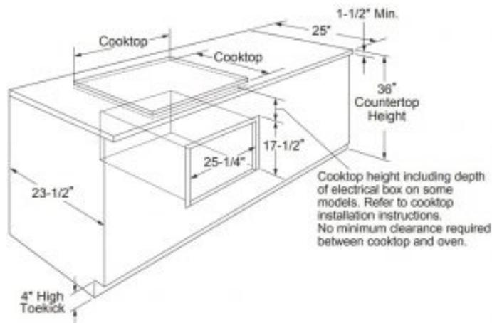
Gas or electric cooktops may be installed over this oven. See cooktop installation instructions for the cutout size. See the label on top of the oven for approved cooktop models. This oven requires a separate, properly grounded 15-Amp, 120-Volt, 60Hz power supply. The cooktop requires a separate power supply. Use a 36 or wider base cabinet.
