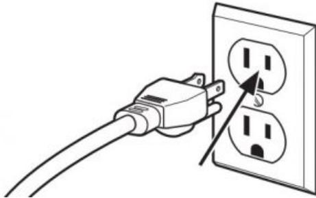
This appliance must be grounded. In the event of an electrical short circuit, grounding reduces the risk of electric shock by providing an escape wire for the electric current.
