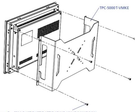
4-M4x8L Screws For FPM-D12T/D15T/D17T/D15W/D18W/D21W/D24W
