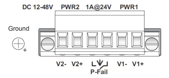
• Wire Gauge: 12-24 AWG (3.31 - 0.205 mm2).
