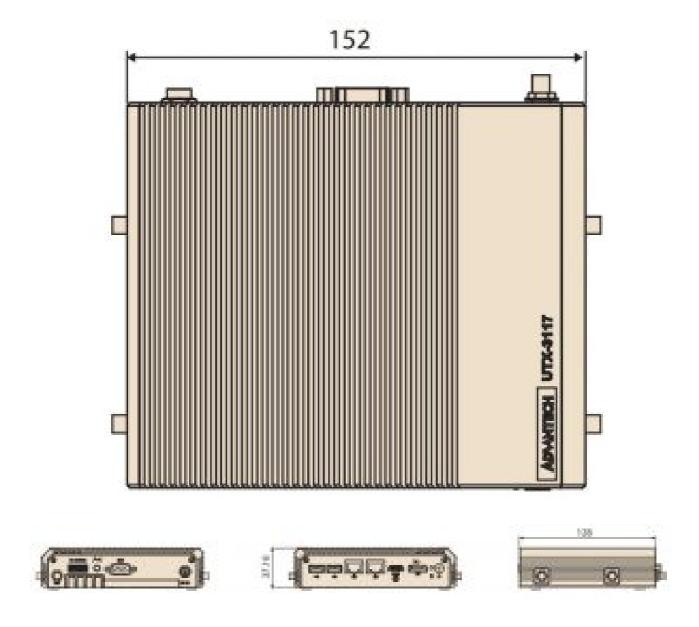
Front Panel External I/O Mechanical Layout/Drawing
