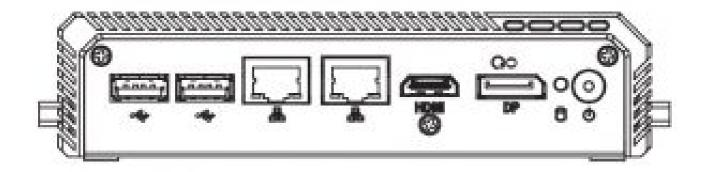
Rear Panel External I/O Mechanical Layout/Drawing
