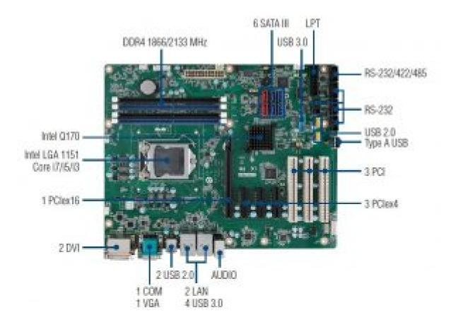
fSupports Intel® 6th/7th generation Core™ i7/i5/i3/Pentium®/Celeron® processor with Q170 chipset
