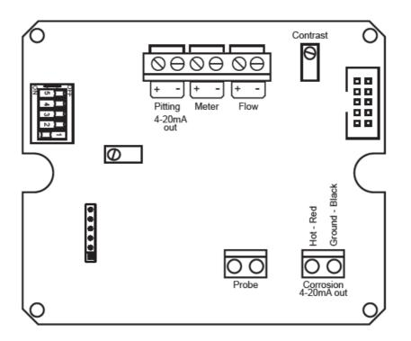
Note: The 4-20mA output has 12 Vdc on the loop.
