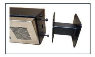
3. Run network cable (CAT5 or better) from POE+ switch or injector through bracket arm in direction shown, then attach bracket arm to load bearing ceiling supports using mounting hardware appropriate to the facility building materials. Note orientation of bracket arm to align viewing direction of clock in hallway or room.
