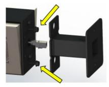
2. Pull ethernet cable from the wall through the bracket arm. Attach bracket arm to wall using mounting hardware appropriate to the facility building materials. Note keyhole orientation with narrow channel of keyhole at bottom.
