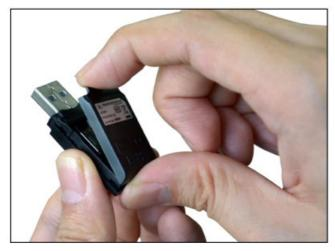
3. Remove the cover completely to insert/remove the SIM card into/from the reader.
