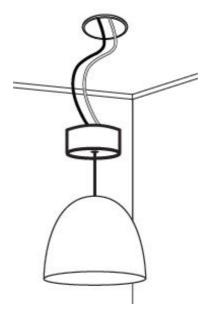
3. Connect the live and neutral wire to "IN" connect the live wire to the right IL] terminal. Connect the neutral wire to the right IN) terminal. Tighten the clamping screws.
