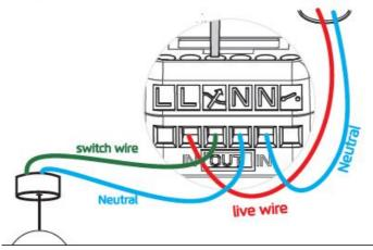
5. Wall installation Remove the existing wall switch This receiver Is a replacement for the existing wall switch and it is not suitable if the existing light switch is interconnected to the other light switches for multi way switching. Do not exceed the maximum load: 2300W.
