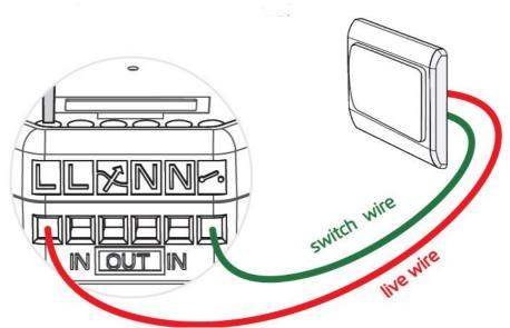
7. If the light is controlled by the live wire and the neutral wire: Connect the live wire to the left IL] contact, Connect the neutral wire to the left IN) or right [N] contact, Connect the switch wire to the [.,...,].
