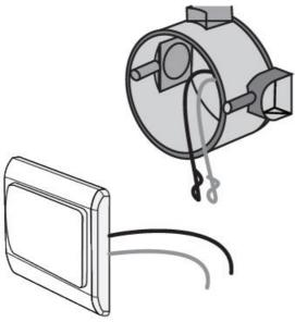
6. Connect the live wire and switch wire: Connect the live wire to the [L] contact. Connect the switch wire to the [.,,.., I contact. Tighten the clamping screws.
