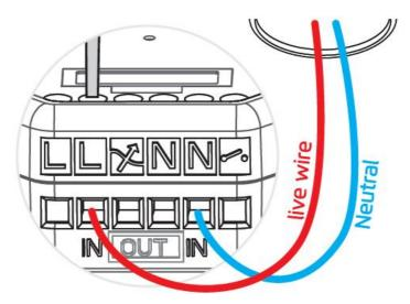
4. Connect 2 wires to "OUT" 2 wires to the Inner 1-,,t: I and [N] contact. Tighten the clamping screws.
