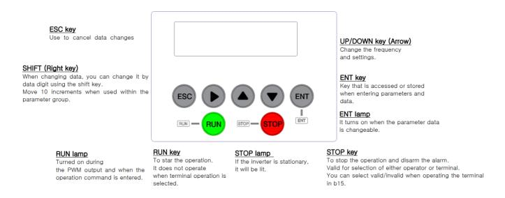
Figure 4-1 LCD Keypad description
