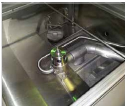
Showing spray arm base & transfer tube
