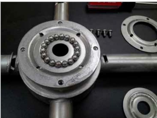
Top race removed, ball bearings for replacement
