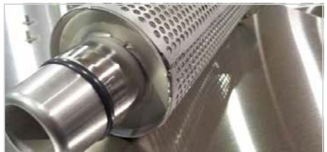
Pump filter and drain plug, note O-ring seal
