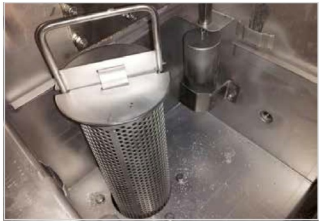
Pump filter in drain sump
