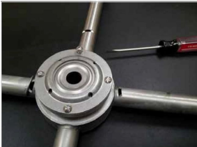
Remove 4 screws and lift top shell
