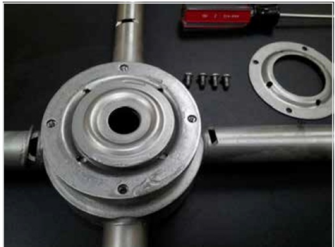
Remove top shell, exposing top bearing race
