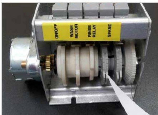
Showing HT-25 cam timer, arrow points to deter cam
