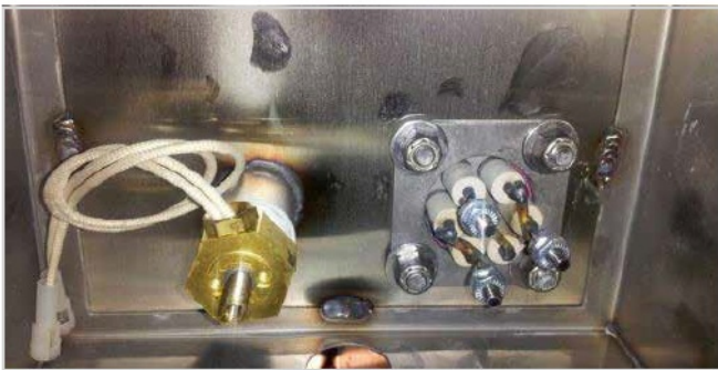
Showing thermostat and sustainer heater terminals*
