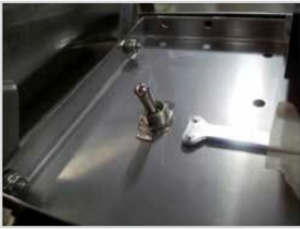
De-lime switch in HT-25 control box
