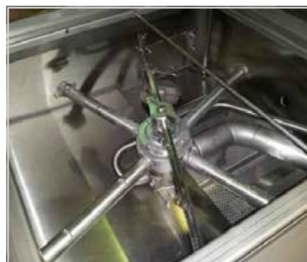
Final rinse arm twisted into transfer tube
