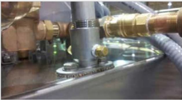
Mixing chamber with two 1/8" pipe threaded port
