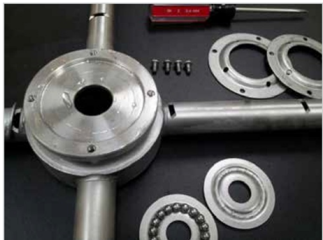
Races are interchangeable, capture shells are also
