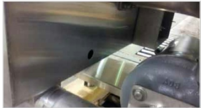
Showing 7/8" detergent probe hole behind pump motor
