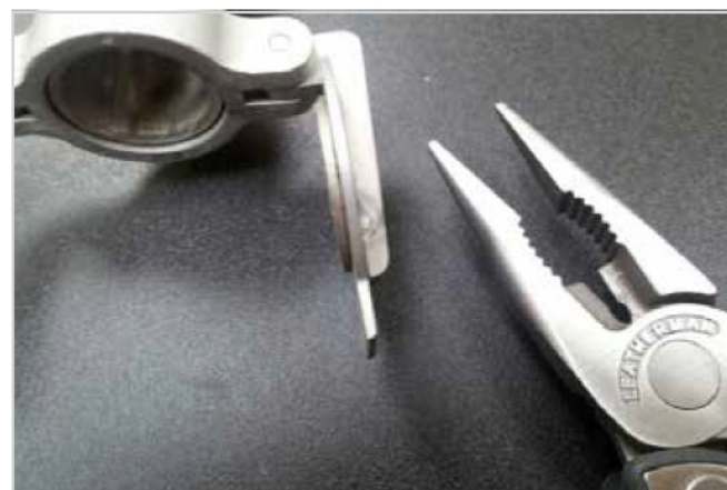
Straighten tab in line with the coin edge to tighten
