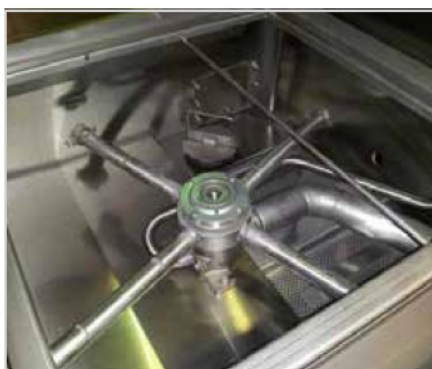
Wash arm w/bearing installed on base
