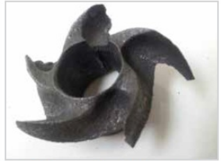
Impeller damaged from high acid solution
