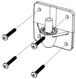
Fit the cabinet half of the bracket to the speaker using the four screws in the centre of the rear of the cabinet.
