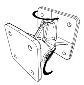
The first stage is to disassemble the bracket so that the cabinet half can be fitted to the speaker and the wall section attached to the wall. A 4mm Allen Key is required. If adjustment is only required in one plane, vertical or
