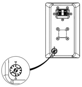
Ensure that the sum of all speaker taps does not exceed the amplifier's rated power output.
