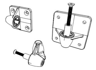
Fit the wall bracket in the appropriate orientation for horizontal or vertical adjustment. Fixings appropriate for the wall surface and weight of the cabinet must be used to ensure a safe and secure installation.
