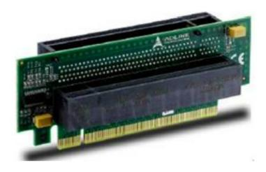
Insert the adapter card into the PCle x16 slot of the Express-BASE7 carrier board as shown below.
