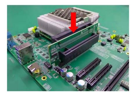
Insert PCIe x8 cards as required into the PCIe x8 slots of the adapter card.
