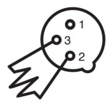
Termination reduces signal errors and avoids signal transmission problems and interference. It is always advisable to connect a DMX terminal, (Resistance 120 Ohm 1/4 W) between PIN 2 (DMX-)
