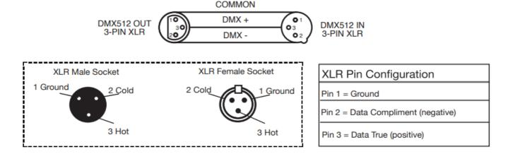
**Special Note Line Termination:** When longer runs of cable are used, you may need to use a termi-nator on the last unit to avoid erratic behavior. A terminator is a 110-120 ohm 1/4 watt resistor which is connected between
