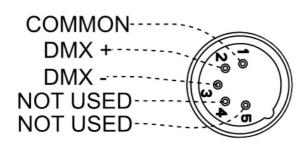
**Special Note:** Line Termination. When longer runs of cable are used, you may need to use a termi-nator on the last unit to avoid erratic behavior. A terminator is a 110-120 ohm 1/4 watt resistor which is connected between pins 2 and 3 of a male XLR connector (DATA + and DATA -). This unit is inserted in the female XLR connector of the last unit in your daisy chain to terminate the line. Using a cable terminator (ADJ part number Z-DMX/T) will reduce the risk of erratic behavior.
