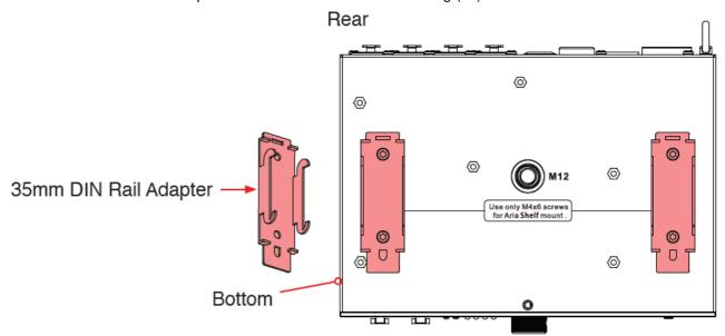
2. Mount the NET 4 by aligning the 35mm DIN Rail Adapters with the slots on the 35mm DIN rail. Slide the NET 4 onto the rail until it clicks or locks into place securely.
