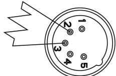
When using longer runs of cable, one may need to use a terminator on the last unit to avoid erratic behavior. A terminator is a 110-120 ohm 1/4-watt resistor, which connects between pins 2 and 3 of a male XLR connector (DATA + and DATA -). Insert this unit into the female XLR connector of the last unit in your daisy chain to terminate the line. Using a cable terminator (ADJ part number Z-DMX/T) will decrease the possibilities of erratic behavior.
