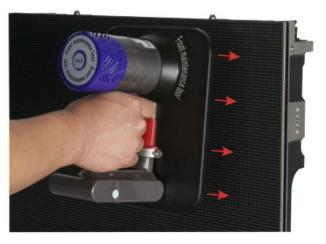
Detach the safety cable for the LED module that you wish to remove. The above left image, for example, shows the location of the safety cable for the upper left LED module. Next, gently press the cusioned face of the vacuum tool to the front of the LED module, as shown in the above right image, and press and release the trigger. Please note that you do not need to continuously hold the trigger to maintain suction.
