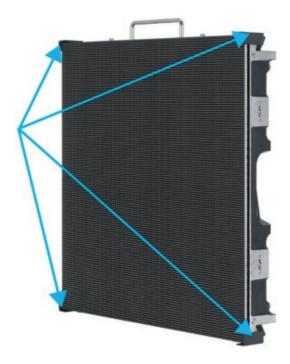
The integrated corner protectors rotate out of their respective housing pockets to protect the cor-ners during storage or transpotation (below right). During installation, these corner protectors can be rotated back into their housing pockets to allow for the fitment of adjacent panels (below left).
