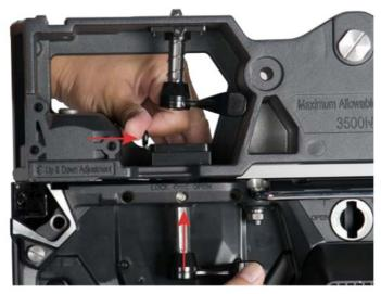
3. Release latch to hold the vertical connector, and twist vertical connector the left to lock
