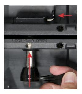
3. Release the latch, then lock the panel in place by twisting the vertical connector lever to the left, towards the direction marked "LOCK".
