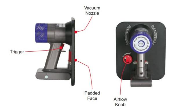
The airflow adjustment knob can be rotated to adjust the amount of vacuum suction force exerted by the tool. Turn the knob clockwise to increase suction force, or counter-clockwise to decrease suction force.
