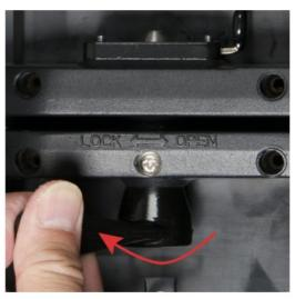
4. To unlock, twist the vertical connector lever to the right, towards the direction marked "OPEN". The locking post will then drop out of place. Press the latch to the left if needed to help release the locking post.
