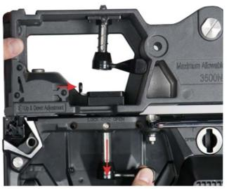
4. To unlock the vertical connector, rotate the lever to the right (counter-clockwise), then press the spring-loaded locking latch inward. The vertical connector will then drop open.
